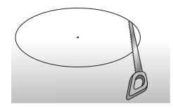
You should wear protective equipment such as Safety Glasses and mask where possible, as dust and debris may fall whilst cutting. Hold the middle of the circle you are cutting when nearing the end to stop the panel falling out.
