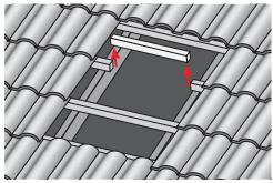
Gently mould the corrugated flashing at the front of the Light Tunnel to match the profile of the tiles
