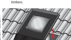
Lower the Light Tunnel into position.
