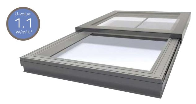
Operated by concealed 24v electric chain link actuators, Signature's Sliding Flatglass rooflights are ideal for providing natural ventilation and roof access, especially in areas where high wind loadings may occur, making a hinged rooflight unsuitable.
